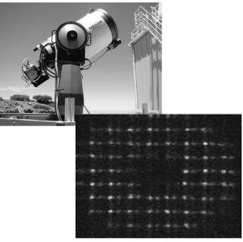
Slope Detection and Ranging (SLODAR) double star technique using the 860 model with 2 ms exposure time. The camera is shown at the European Southern Observatory (ESO) site at Cero Paranal in Chile, mounted on a 40cm Schmidt-Cassegrain telescope and operated through Linux. The image shows an example Shack-Hartmann wavefront sensing frame.
