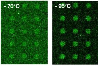
Images of extremely dim LED signal (signal intensity typical of weak luminescence experiments) acquired with iXon<sub>3</sub> 888 at cooling temperatures -70°C and -95°C (water cooling to achieve latter), 120 sec exposure times, sub-region show. The need to push to such deeper cooling temperatures can be readily observed under such extreme low light conditions
