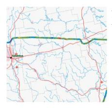
An example of a FALLS® Exposure Analysis for a transmission circuit in eastern Ohio. Areas of higher lightning activity are revealed. This information can help an electric utility to prioritize protection or maintenance.
