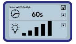
The selection of the background illumination, respectively the time until the automatic shut-down of the same is selected via the button " $\square$ " by actuating the same several times. Using the button " $\square$ , you can adjust the intensity of the illumination, respectively turn the same completely off. Activate and store your settings by actuating the button " $\square$ ". After activation, the symbol  $\square$  will appear in the upper right hand corner of the display.
