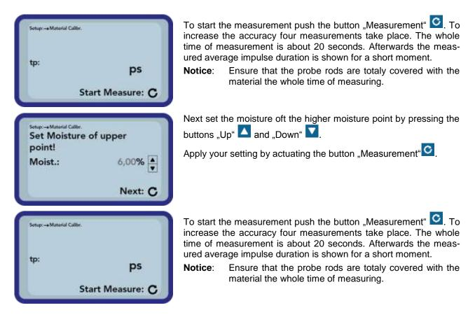
Attention: If you choose "SAVE" at the end of calibration, the stored calibration inside the probe is overwritten! The only possibility to get back the original calibrations is to connect the probe with a RS485 adapter (for example SM-USB) to the PC. Also you need the software PICO-Config.
