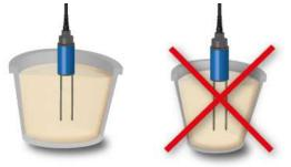
• The filling depth of the bucket has to exceed the rod length by minimum 5cm
