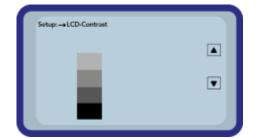
Change the contrast by actuating the button  $"Up" \land$ , respectively "Down"  $\checkmark$ . Set the contrast that you can realize the whole grayscale on the diagram. Activate and store your settings by actuating the button "Measurement"  $\bigcirc$ . After activation, the symbol  $\square$  will appear in the upper right hand corner of the display.
