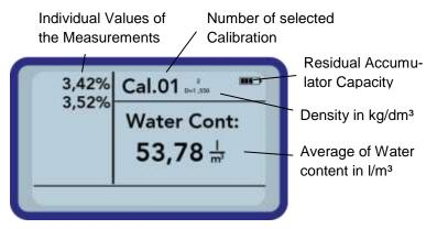
In order to delete the measurement series, actuate the button "Down" **M**.
