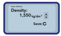
Adjust the density of your material by actuating the buttons "Up" and "Down" . Confirm your setting by pressing the button "Measurement" . You will then automatic get back to the measurement screen. Leave the setting without changing the density by pressing the button "Settings" .
