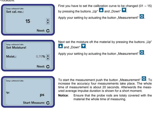
Attention: If you choose "SAVE" at the end of calibration, the stored calibration inside the probe is overwritten! The only possibility to get back the original calibrations is to connect the probe with a RS485 adapter (for example SM-USB) to the PC. Also you need the software PICO-Config.
