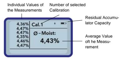
In order to initiate a measurement, shortly press the button "Measurement" **O**. The measurement will com-
