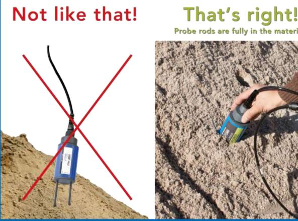
Probe rods are fully in the material.
