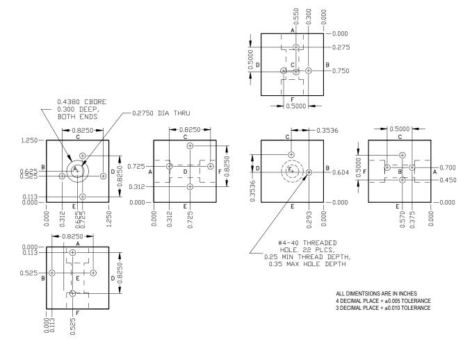
The #4-40x1/2" screws attach your accelerometer(s) to the block. The 1/4-20 or M6x1 screw attachs the block to your work surface.
