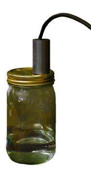
Apogee oxygen sensor mounted in a sealed chamber over water. For measurements in environments where relative humidity is 100 %, sensors should be calibrated in conditions where relative humidity is 100 % in order to account for any humidity effects on sensor electronics.
