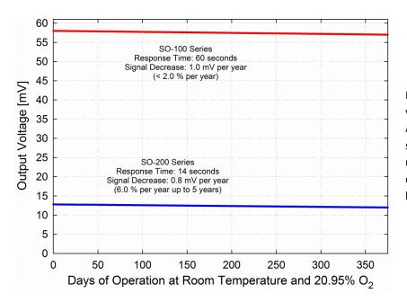
Long-term stability (output voltage decrease over time) of Apogee SO-100 and SO-200 series oxygen sensors. The response time and signal decrease for both series are also listed.
