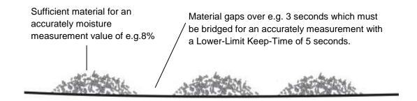
The following parameter setting in mode CA fits a high pass filtering for bridging material gaps.
