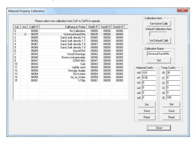
The desired and possibly altered calibration curve (Cal1. .15) which is activated after switching on the probes power supply can be adjusted with the button "**Set Default Calib**".
