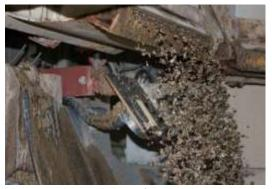
Gravel or grit could have so much water, that free water can flow above the probes's surface. E.g. the maximum moisture content of gravel with 2-8mm grain size lies at 3.5%. For gravel with 8-32mm grain size the maximum lies at 2.5%.
