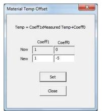
In the menu "Calibration" and the window "Material Temp Offset", a zero point offset can be adjusted for the material temperatur sensor which is installed inside the SONO probe. In this example a temperature deviation of +5° C is produced by inside self-warming of the SONO probe. The correction value -5 can be setted in the Coeff0 window.
