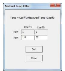
The example shows the parameters for displaying the temperature in the unit: Degree Fahrenheit.
