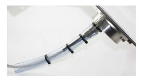
Alternatively, the included shrink sleeve over the cable can be used. After installation of the SONO-probe and connection of the MIL-connector, the shrink sleeve can be shrinked with a hot air blower.
