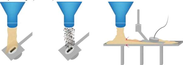
Installation of the SONO-VARIO for measuring sand, gravel and grit, under a silo valve or on a conveyor belt. Dependent on material, it is important to find the suitable angle of the mounting plate. It should be not too steep, but also not too flat and the flowing material should cover the probes surface completely during flowing. But material should also not accumulate.
