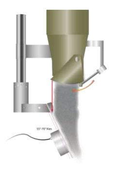
Sand: Angle baffle plate 45° to 55°
