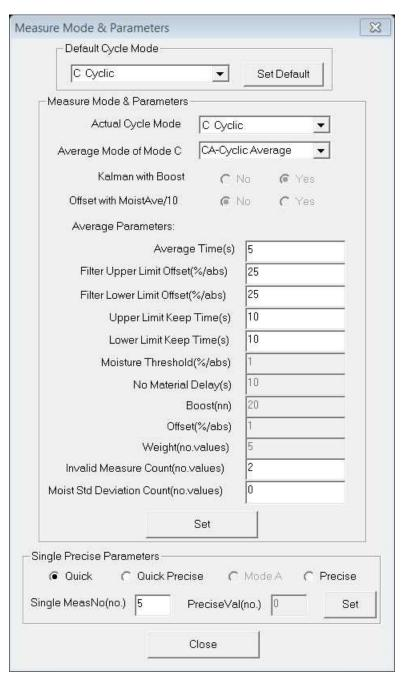
By selecting the operating mode, the SONO probe can be set up to different measurement modes, e.g. for averaging values from several single measurement values, for performing a filtering or performing other functions (see chapter "Measurement mode configuration" in this manual).
