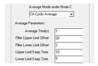
The Filter Upper-Limit is here deactivated with a value of 20, the Filter Lower-Limit is set to 2%. With a Lower-Limit Keep-Time of 5 seconds the average value will be frozen for 5 seconds if a single measurement value is below the limit of 2% of the average value. After 5 seconds the average value is deleted and a new average value building starts. The Keep-Time function stops if a single measurement value lies within the Limit values.
